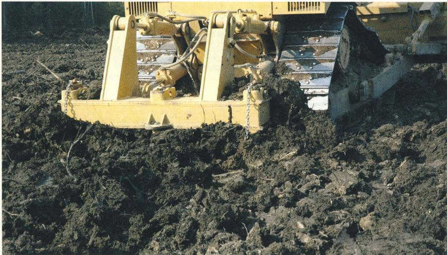
FIGURE 4: SOIL PILED UP IN FRONT OF THE TOOLBAR CAN OFTEN BE CLEARED BY TEMPORARILY RAISING THE TOOLBAR A SHORT DISTANCE.
