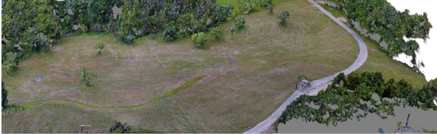
Figure 1. UAV (DJI Phantom 4) captured 3D image (no glare; color enhanced), leading to a recently forest-cleared strawberry field. UAV flight height was 60 metres above ground level (agl) in reference to a fixed take-off point. Image overlap was > 60 per cent along planned flight path. Flight time was 60 minutes on July 28, 2017, starting at 12:30 p.m. Weather was partly cloudy. Resulting image resolution: 0.02 m. 3D image and DEM producing software: Agisoft Photoscan Professional Version 1.3.2 (64 bit; Agisoft 2017). Latitude 45.369°; Longitude - 66.257°.
