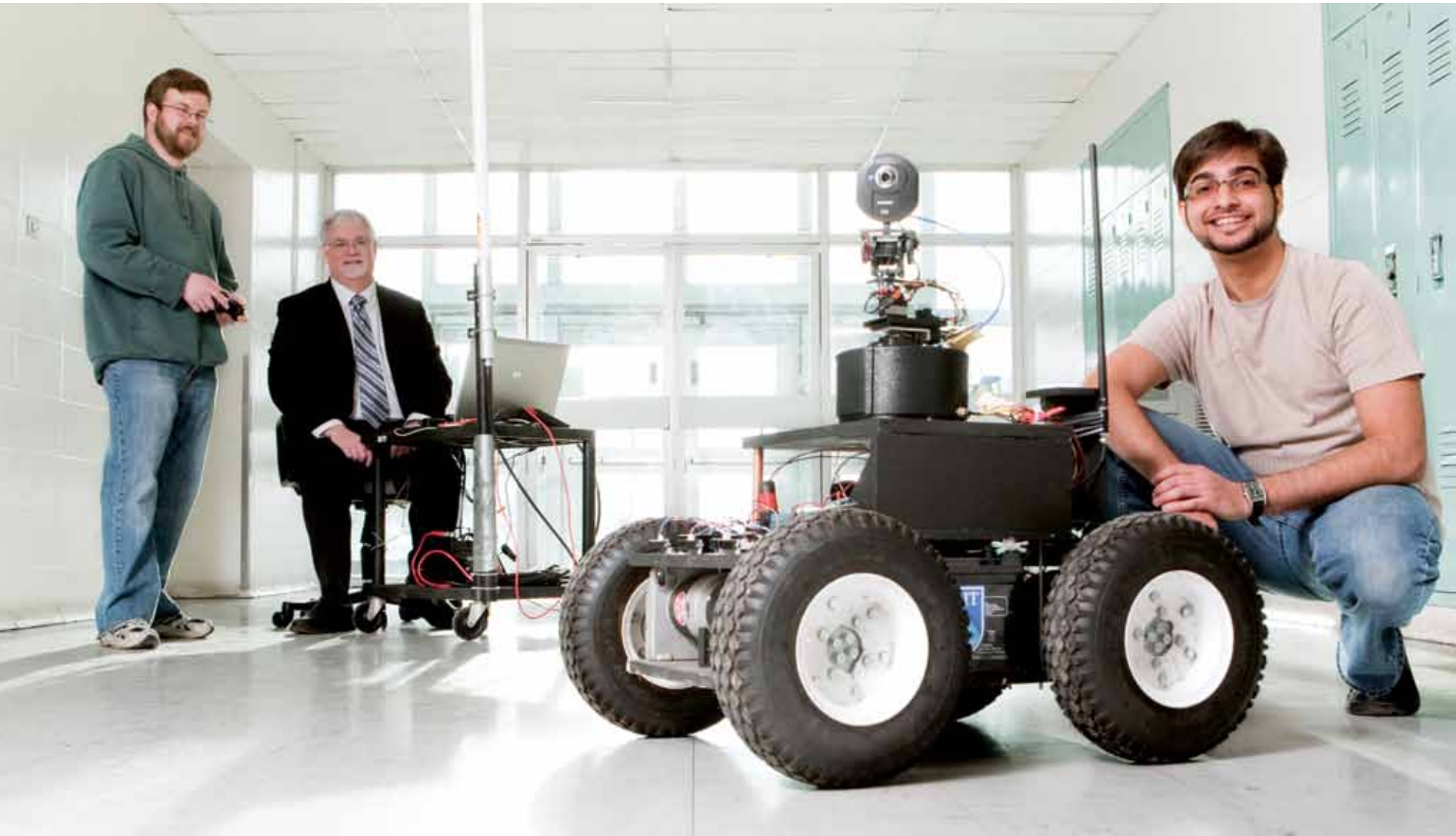
Left, Woody can reach speeds of 16 km/h and climb curbs, making it a tactical asset in police activities.
