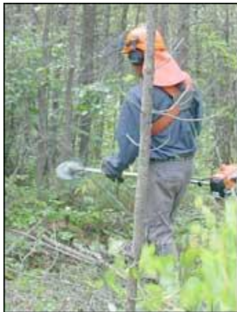
Figure 4. Brushsaw being used to control woody brush.
