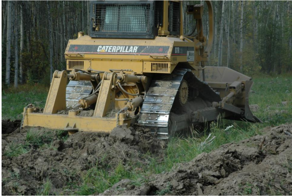
Figure 2. Ripplow decompaction treatment results in substantial disturbance.
