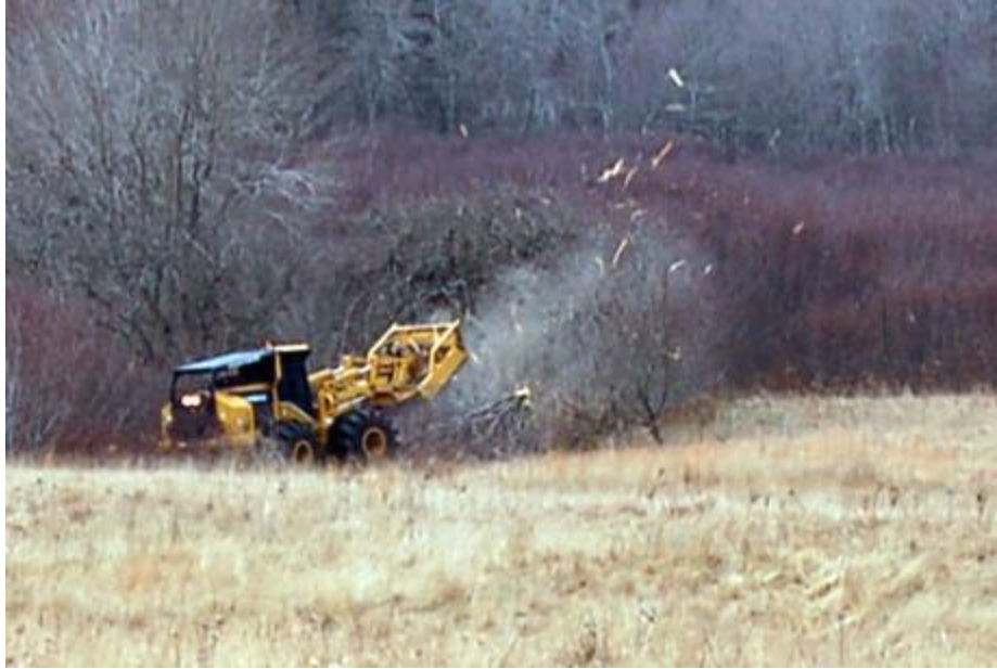
Figure 6. Hydraulic powered self-propelled mower mowing large brush.
