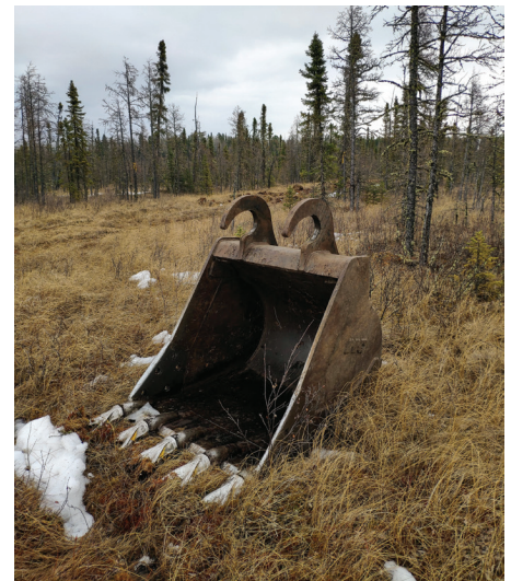
Figure 2B. A digging bucket (1 yard) equipped with frost-teeth.
