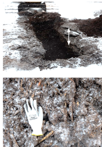
Figure 2. Thick wood chip overburden (top) and close-up of the fine wood chips (bottom).
