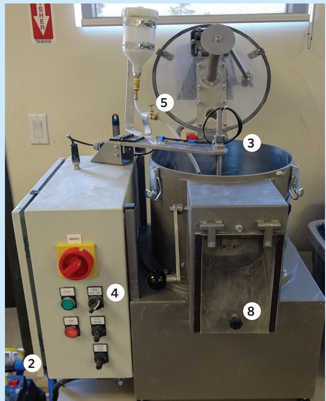
Figure 4. Seed pelleting machine. Numbers indicate selected steps in above list.
