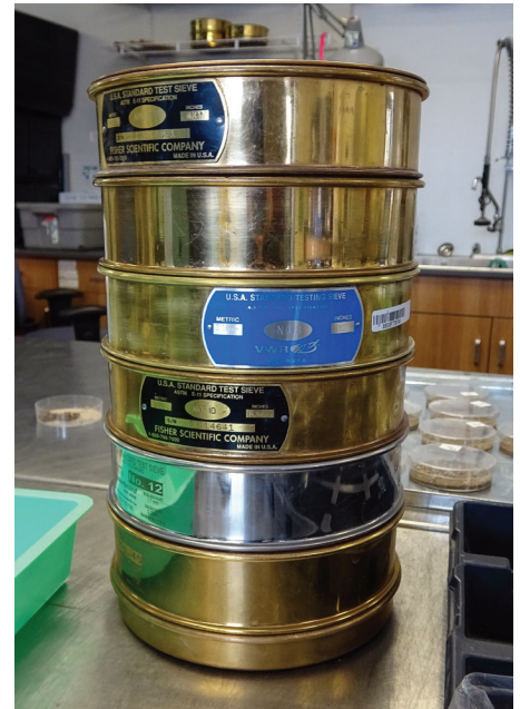
Figure 2. Sieves for sorting seed pellets by size.
